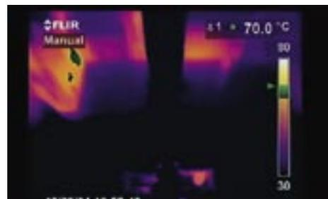
gearbox monitoring: exceeding the threshold
