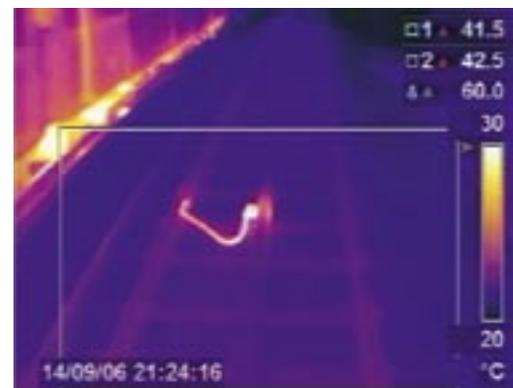
surveying traction supply: defective jumper
