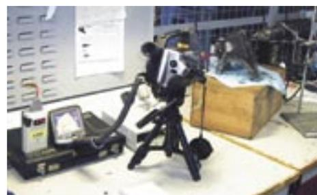
gearbox monitoring: IR camera setup
